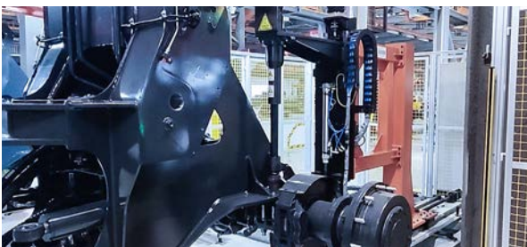
Vision-Guided Bolt Tightening
